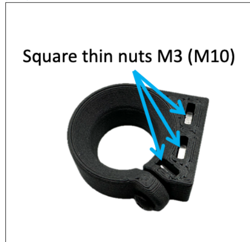
Figure 4-8 Square nut position Thumb-Stick-Lever (P32).
