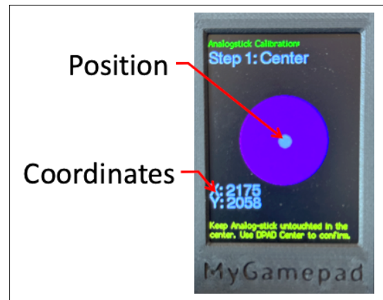
Figure 2-13 Analog stick calibration step 1.
