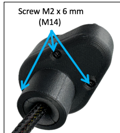
Figure 4-36 Inserting screws from the bottom side.
