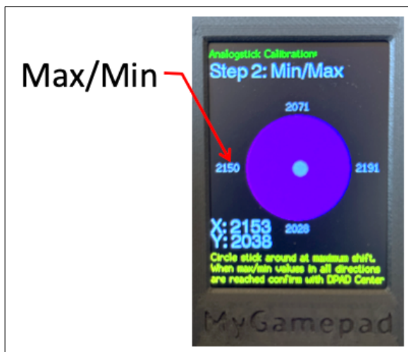
Figure 2-14 Analog stick calibration step 2.
