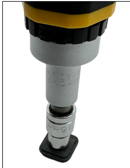
Figure 4-15 Using a 6 mm nut to press the key parts together.
