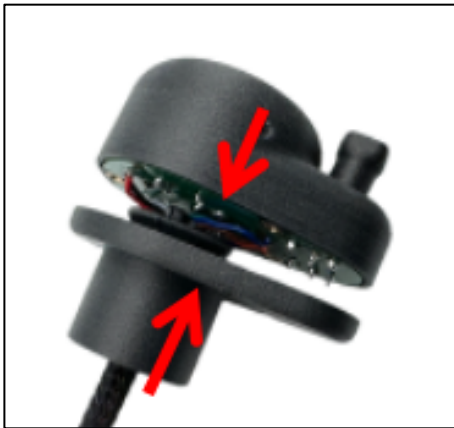
Figure 4-35 Sliding the thumb stick housing together.
