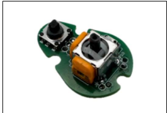
Figure 4-32 Placement of components on the Thumb-Stick-PCB.
